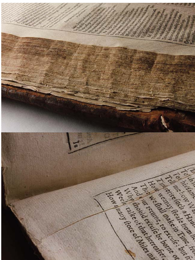
Features triggering further research: suspected drawknife trim marks on fore-edge of textblock (above) and papermaking flaw (below). The Bodleian Libraries, University of Oxford, Arch. G c.7, Tragedies p. 381
