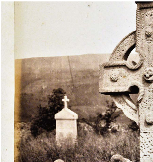
Loss of image density and discolouration to the edge of this albumen print (Anon. Irish Cross, Kilkispeen, County Tipperary 1866) arising from drum-mounting the print with unrefined gelatine
