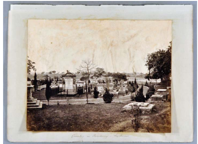
This Samuel Bourne albumen print (Neg. 1064 Cemetery in Residency Lucknow 1860s) clearly shows image silver degradation arising from the caoutchouc adhesive
